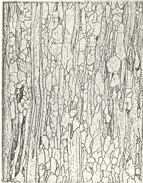
FIG.13 AT 597°C FOR 2 MINUTES (ROCKWELL 30T 52.6) -150 X- FIG.14 AT 540°C FOR 42 MINUTES (ROCKWELL 30T 51.9)
